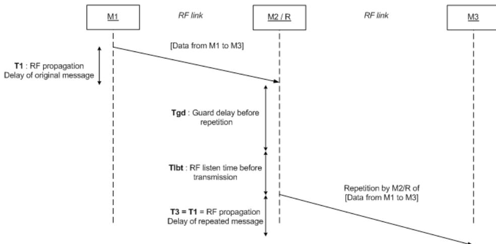
**Minimum RF overall message propagation delay = 2\*T1 + 1\*Tgd + 1\*Tlbt**
