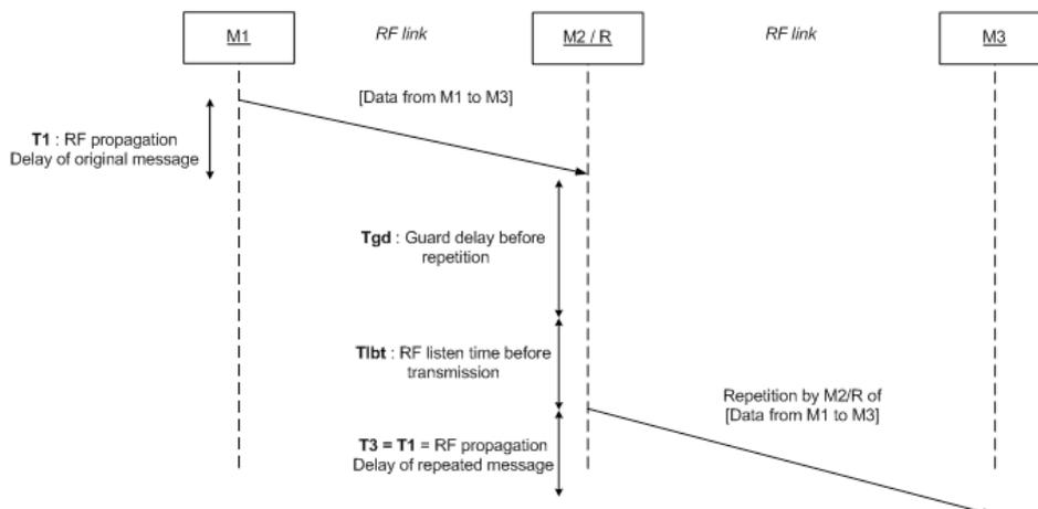
$$\text{Minimum RF overall message propagation delay} = 2 \cdot T1 + 1 \cdot Tgd + 1 \cdot Tibt$$
