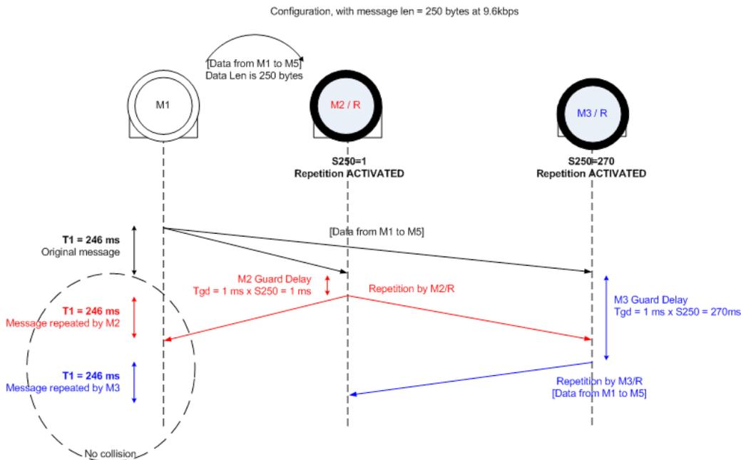
Elements of calculation of RF propagation time of a frame: :
